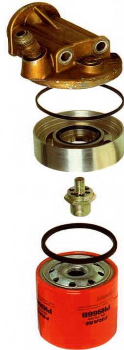
Remove the canister and old oil filter. Remove the rubber seal which sits in a groove in the filter head and clean out the groove thoroughly. Place a tommy bar through the hole in the central mounting boss (this is the steel part into which the canister retaining bolt screws) and unscrew the boss. Remove the boss, the splash plate (if fitted) and the felt washer which sits under the splash plate.
